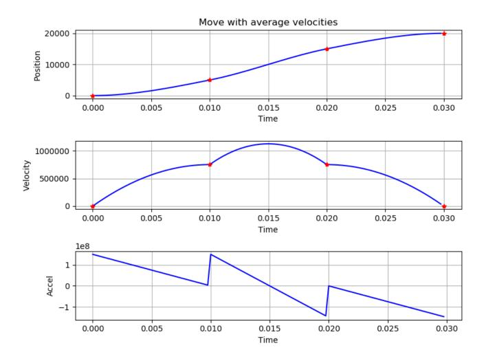
This is a much smoother looking move then the previous one. As before, the position and velocity points are hit exactly by the drive. The acceleration still changes abruptly at the start of each point, but the change is less severe then in the previous example.
