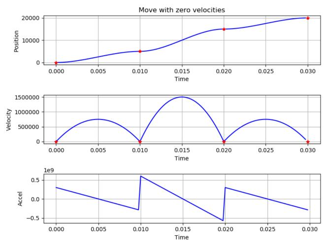
In the position and velocity graphs the points given by the master are identified with a red asterisk. The blue line shows the interpolated data between the points. Notice that the drive is correctly moving between the given data points and that position and velocity are continuous. The interpolated acceleration value moves linearly between points, but jumps to a new value at the start of each segment.
