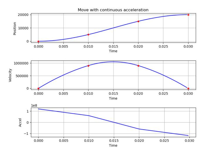
As always, the positions and velocities (marked in red) are hit exactly by the interpolation calculations. The accelerations happen to be continuous between the points due to the way the velocities were calculated for this move.
