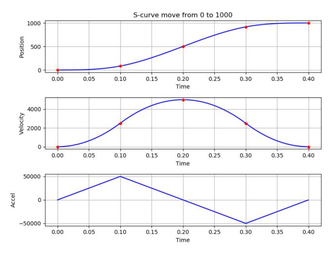
One could calculate slightly more complex s-curve moves which limited the maximum velocity and/or acceleration to desired values. Such moves would consist of more segments then the simple s-curve move shown above, but any such move can be easily described as a set of PVT points.
