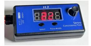
For the model above the Select button changes the circulation patterns, the Pulse Width button controls the frequency, and the knob controls the speed of the amplitude signal.
