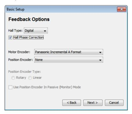
2 Open the Motor/Feedback screen's Feedback tab.
